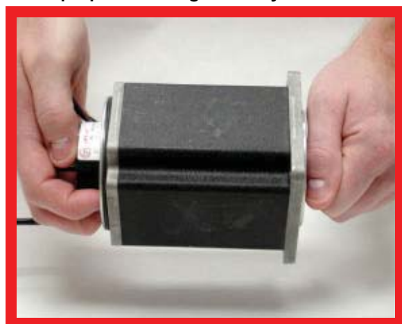
Improper Handling: lifted by encoder
