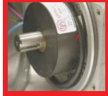
Improper: Run under encoder
