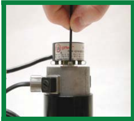
Tightening down the Flex
