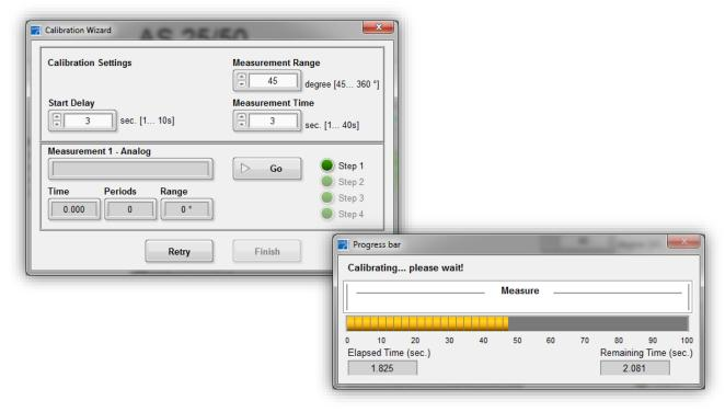
Now immediately start turning the magnetic wheel **in one direction** (in your application) within the time you've entered. When the complete angle is reached and time is finished, the green beacon switch to Step 2.
